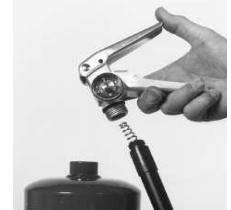
14. Return spring to syphon tube, turn syphon tube clockwise into valve body.
