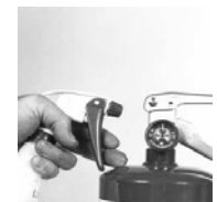
20. Thoroughly check all areas on the unit that may leak pressure. a) welds b) gauge face & threads c) valve body o-ring d) valve stem seat
