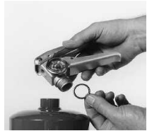
6. Remove body o-ring.
