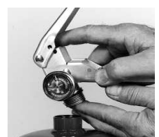
5. Using your finger or a suitable tool, press down on the valve stem located under the discharge handle.
