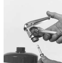
13. Re-insert valve stem assembly into the valve body. Push into place with your finger.
