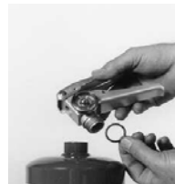
8. Carefully inspect the new Valve Body O-ring and install. Be carefull not to damage o-ring on valve body threads.
