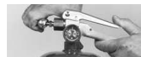
18. Place the pressurizing adaptor into valve outlet. Move regulator to desired pressure (use Dry Nitrogen ONLY). Connect Nitrogen source and allow pressure to felt at valve stem. Push down discharge handle. Nitrogen will be forced around valve stem and down syphon tube. A small bump may be noticed due to the displacement of dry chemical in the syphon tube. Once the gauge on the unit has reached the correct pressure, release the discharge handle. Remove recharge adaptor.
